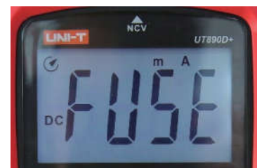
Fuse blowing alarm (mA only)
